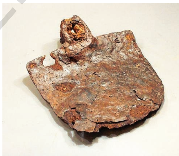
fig-17: Rusting of iron
