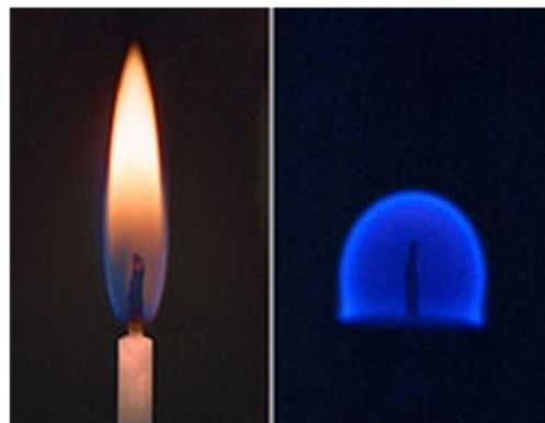
Fig. 17.7 Burning candle in the International Space Station as compared that on the Earth
