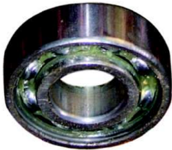
Fig. 12.16 : Ball bearings reduce friction
