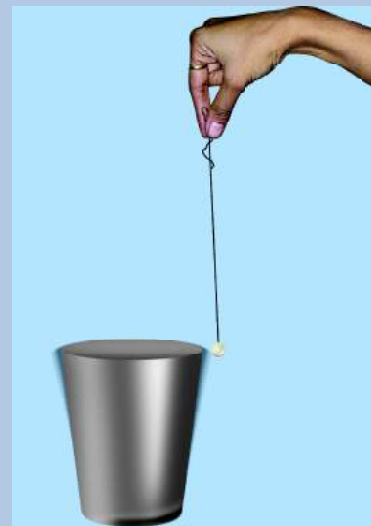
Fig. 13.17 : ThermoCole ball touching the vibrating glass tumbler
