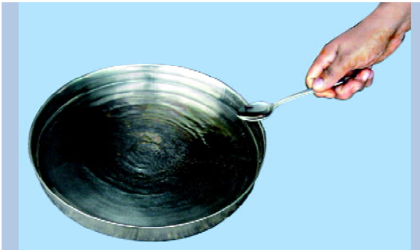
Fig. 13.4 : Vibrating dish produces waves in water
