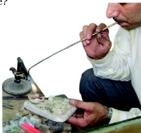
Fig. 6.14 : Goldsmith blowing through a metallic pipe
