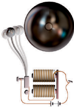
Fig. 14. 20 Circuit of an electric bell
