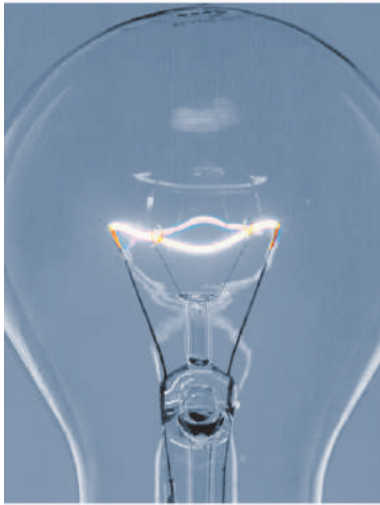
Fig. 14.12 Glowing filament of an electric bulb
