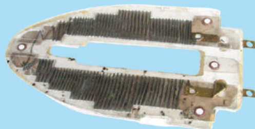
Fig. 14.11 Element of electric iron
