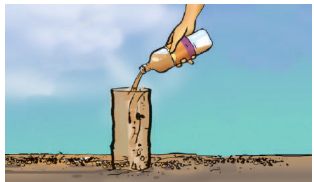
Fig. 9.5 Measuring rate of percolation
