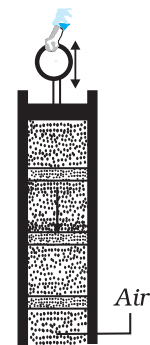
Fig. 15.4 Longitudinal waves (sound) generated in a pipe filled with air by moving the piston up and down. A volume element of air oscillates in the direction parallel to the direction of wave propagation.
