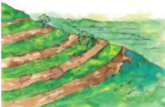
Continuous contour trenches (CCT)
