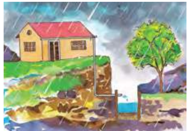
Making rainwater seep into the soil
