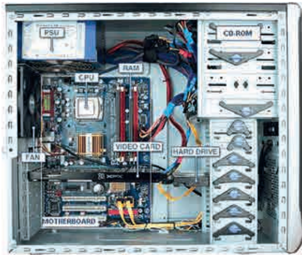
Fig : 3 CPU Internal View
