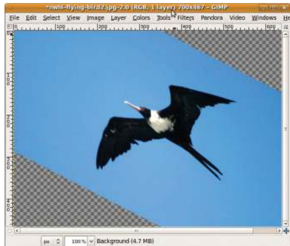
Fig 6.64 : After applying Shear
