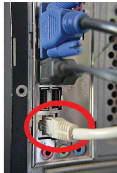
Fig. 5.3 A UTP cable is connected to a computer.
