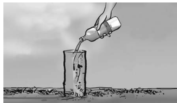
Fig. 9.5 Measuring rate of percolation
