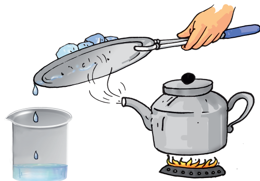
Fig. 5.13 Evaporation and condensation
