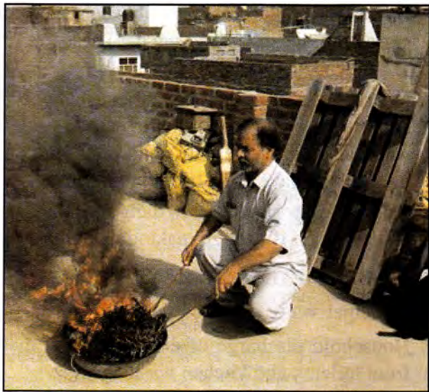
Fig. 19.2 A scrap dealer is burning some electronic waste equipment to extract metals from it. It is a harmful practice which gives out poisonous gases.
