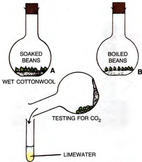
Fig. 7.3 Experiment to show the production of carbon dioxide in germinating seeds.
