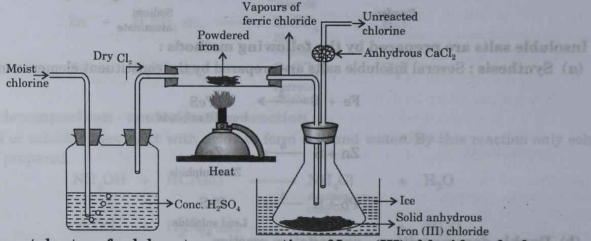
Experimental set-up for laboratory preparation of Iron (III) chloride anhydrous
