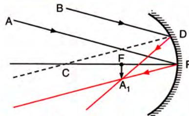
Fig. 7.32 When the object is at far distance
