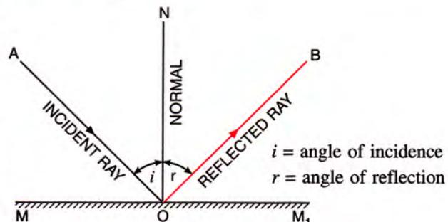
Fig. 7.3 Reflection at a plane surface
