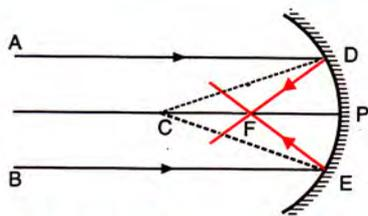
Fig. 7.31 When the object is at infinity
