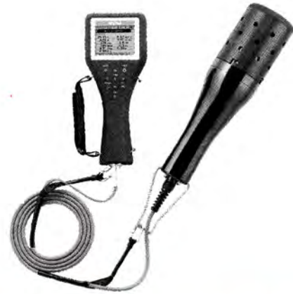
Fig. 9.6 Instrument for measuring dissolved oxygen
