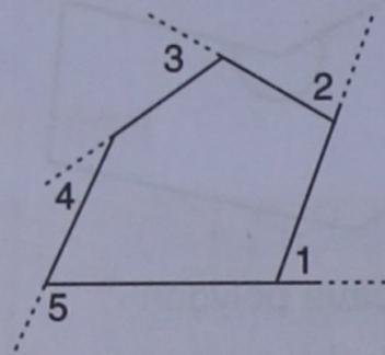
$$[\angle 1 + \angle 2 + \angle 3 + \angle 4 + \angle 5 = 360^\circ]$$
