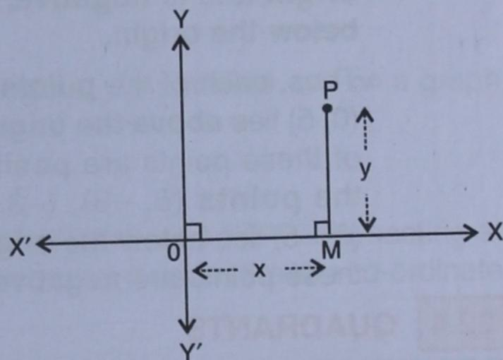
In stating the co-ordinates of a point, the abscissa precedes the ordinate and both are enclosed in a bracket after being separated by a comma.
