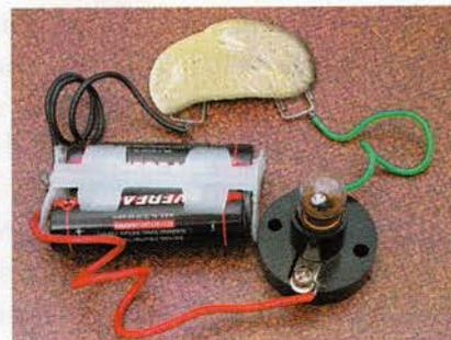
**Fig. 6.4** A metal key conducts electricity but a block of sulphur does not.
