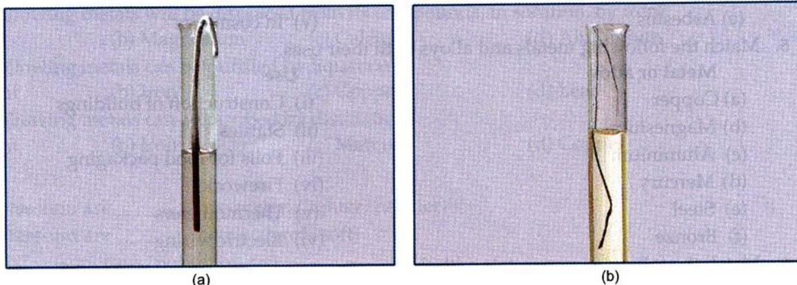
**Fig. 6.13** (a) Aluminium wire dipped in  $CuSO_4$  solution (b) Aluminium wire dipped in  $FeSO_4$  solution. The colour of both the solutions will change.
