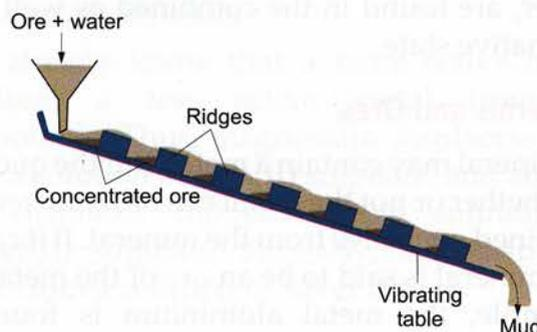
Fig. 6.8 Gravity separation
