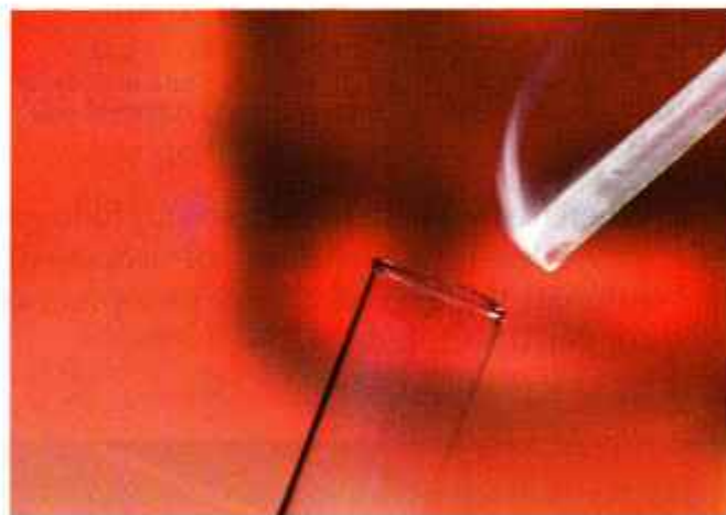
Fig. 5.15 When a glass rod dipped in \text{NH}_4\text{OH} is brought near a test tube containing \text{HCl} , \text{NH}_4\text{Cl} is formed. The solid particles of \text{NH}_4\text{Cl} give white colour to the vapours.
