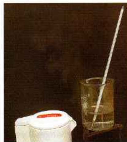
Fig. 5.3 Vapours give out heat while condensing.
