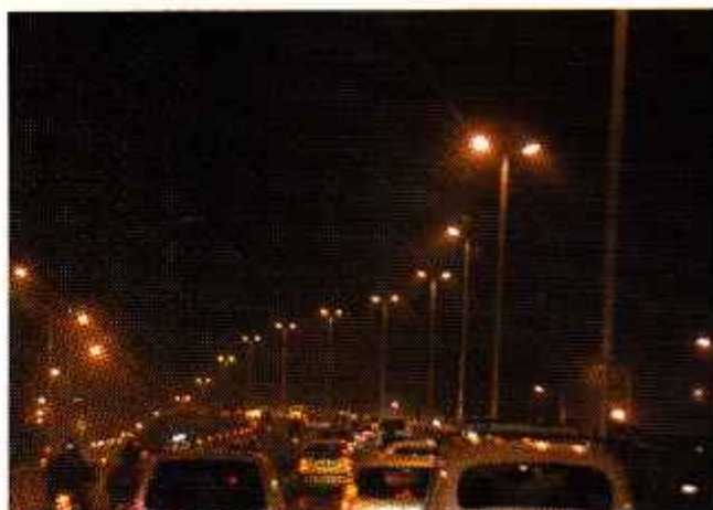
Fig. 4.11 A sodium-vapour lamp gives a golden yellow light due to electron transition in sodium.
