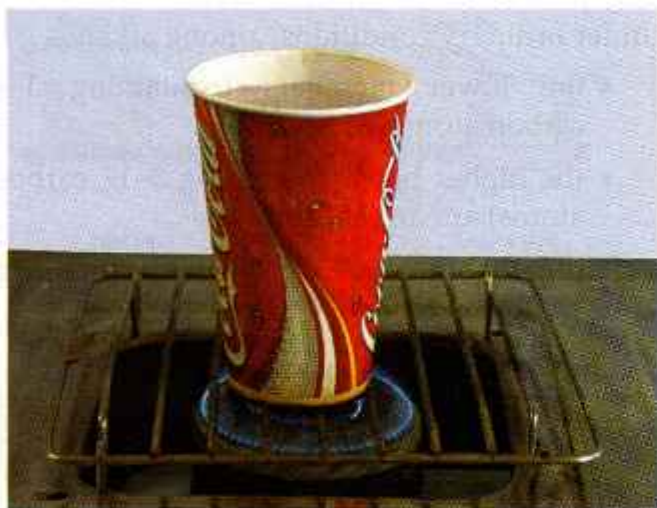
Fig. 3.1 A paper cup containing water does not burn when placed over a flame.
