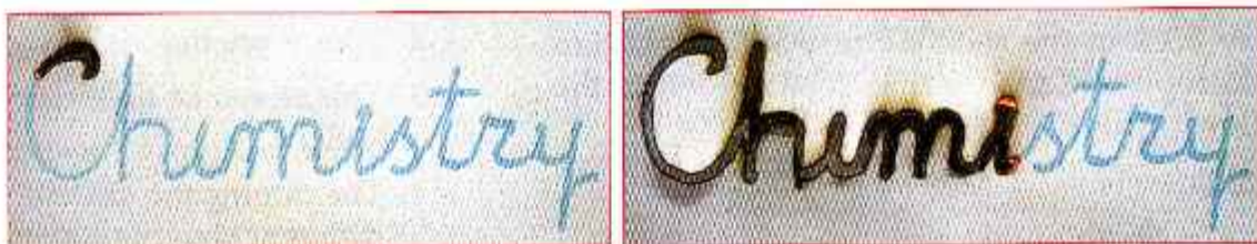
Fig. 3.12 What you have written with potassium nitrate solution burns with a glow.
