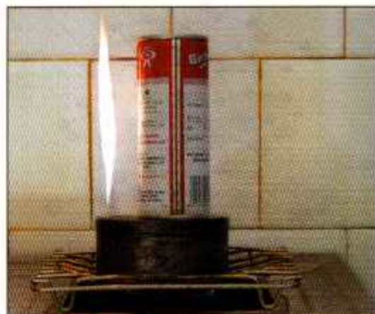
Fig. 2.11 Making wood charcoal at home
