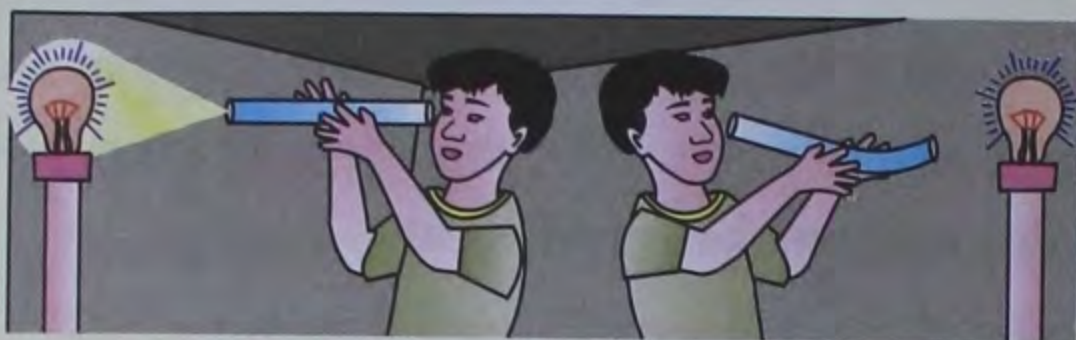
Fig. 5.7 Rectilinear propagation of light
