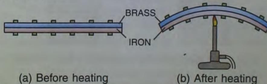
**Fig. 4.16** Different solids expand differently in length
