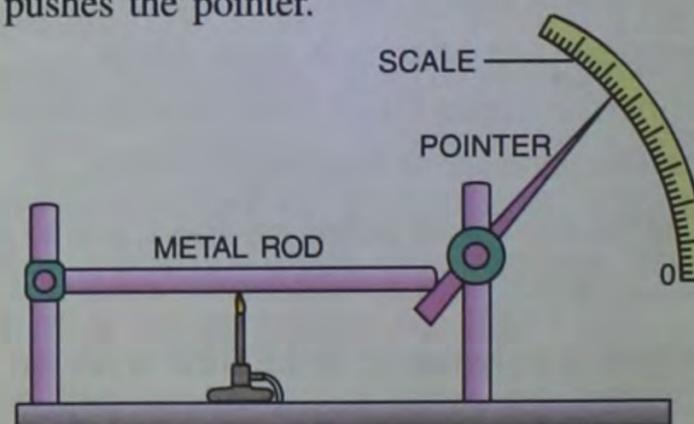
**Fig. 4.10** Metals expand on heating
