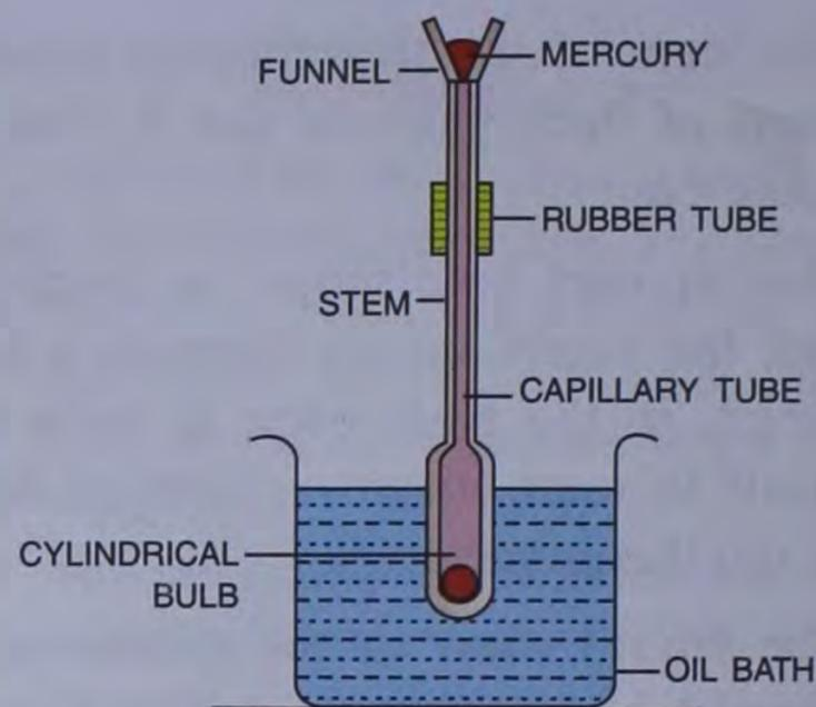
**Fig. 4.4** The capillary tube being filled with mercury
