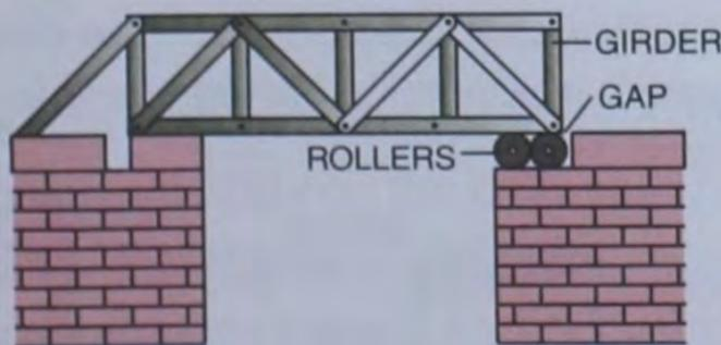
**Fig. 4.12** Gap for the expansion in a bridge
