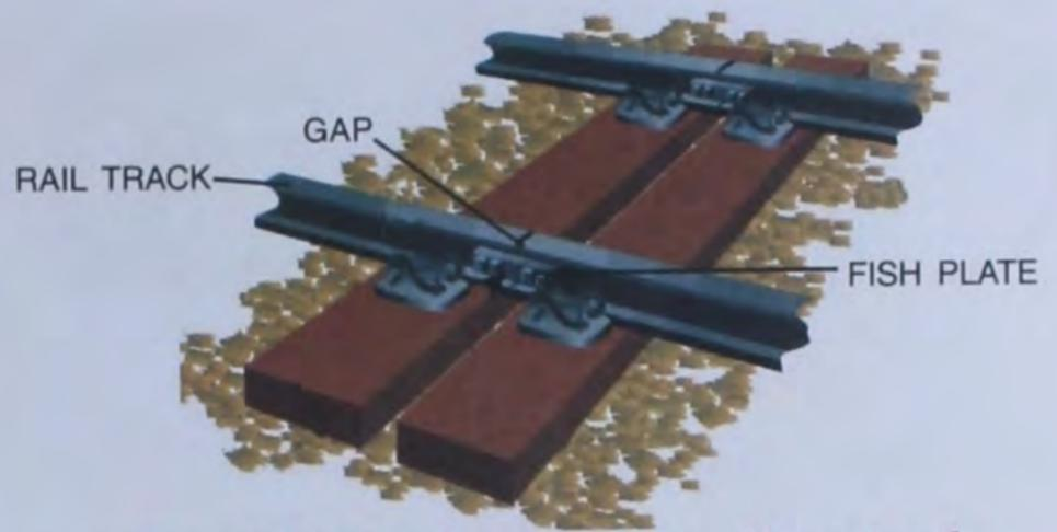
**Fig. 4.13** Gap between the railway tracks
