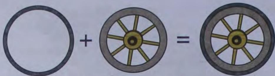
**Fig. 4.15** An iron rim is heated to fit it on a wooden wheel
