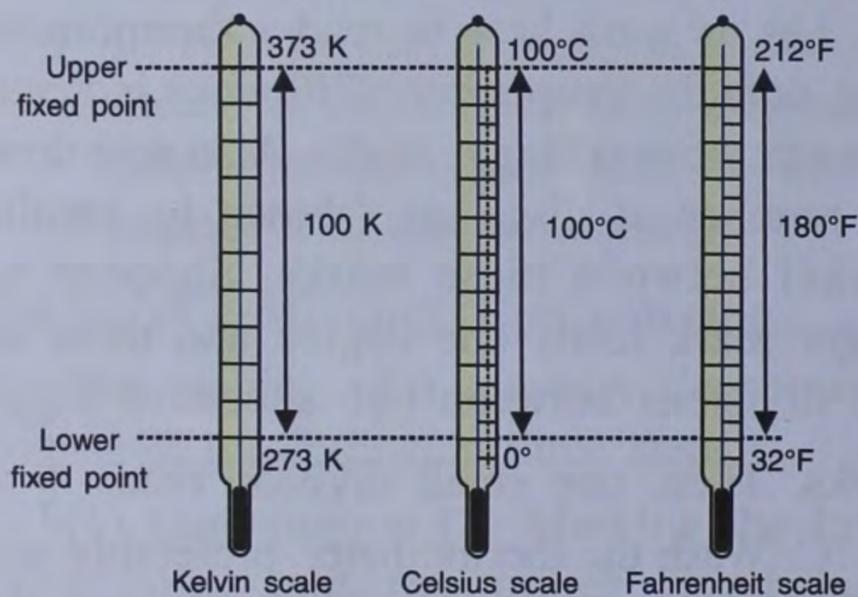
Fig. 4.7 Temperature scales of thermometers
