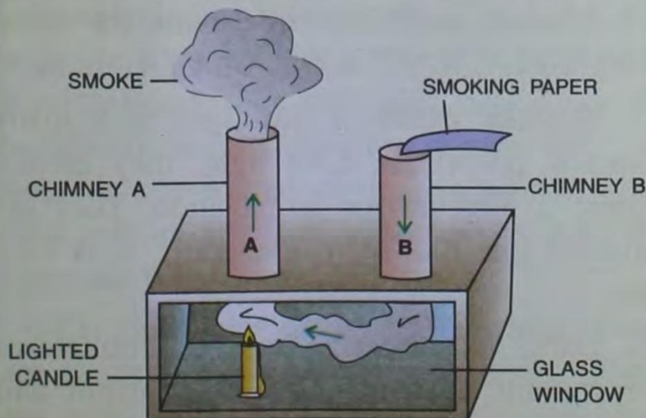
*Fig. 4.23 An experiment to show convection in gases*
