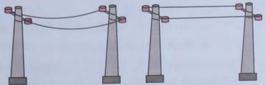
**Fig. 4.14** Electric wires are kept loose for the contraction in winter
