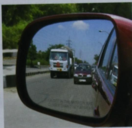
**Fig. 6.20** (a) Convex mirrors produce images that are erect and smaller than the object.
