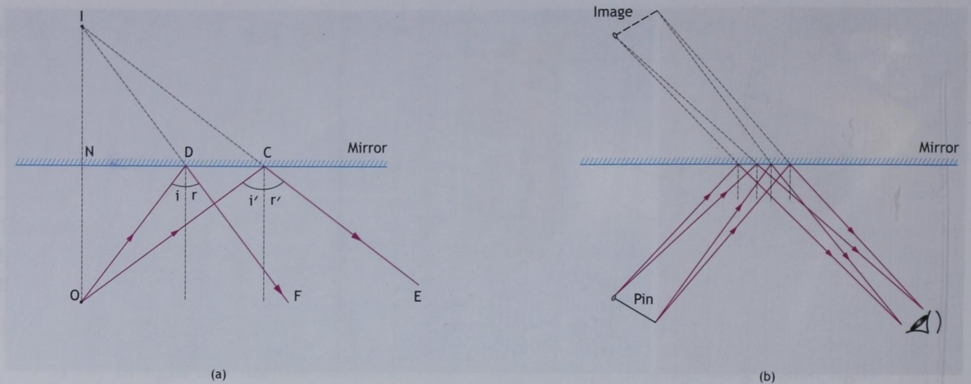
**Fig. 6.6** (a) The image is as far behind the mirror as the object is in front of it. (b) The object and the image are of the same size.
