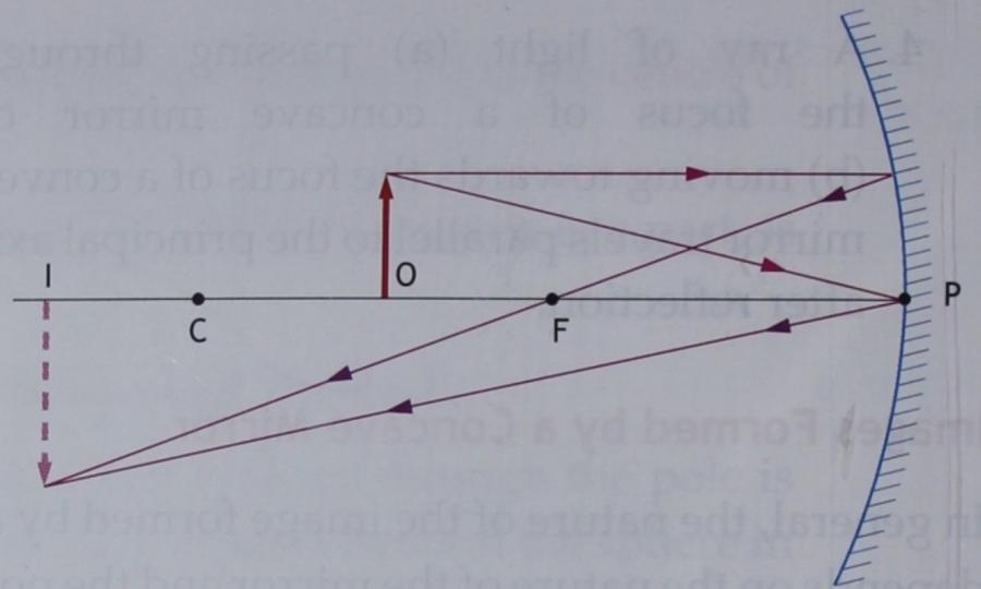
Fig. 6.17 Object between C and F
