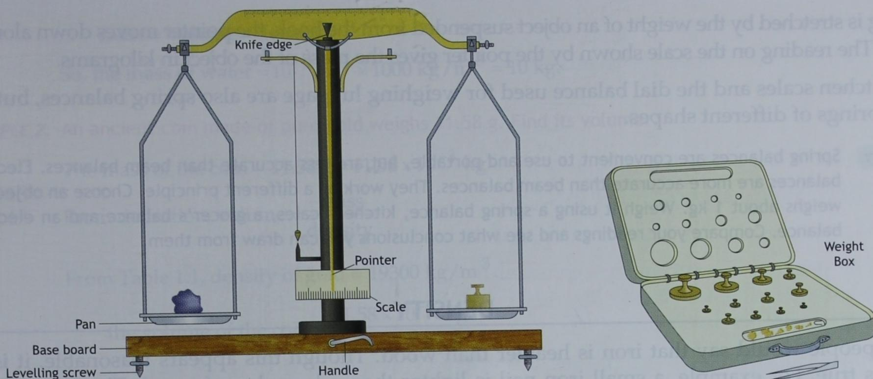
Fig. 1.2 Physical balance and weight box
