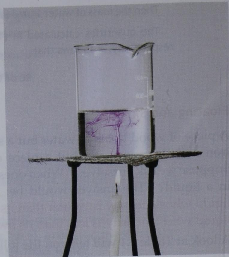
Fig. 1.6 Convection current in a beaker of water
