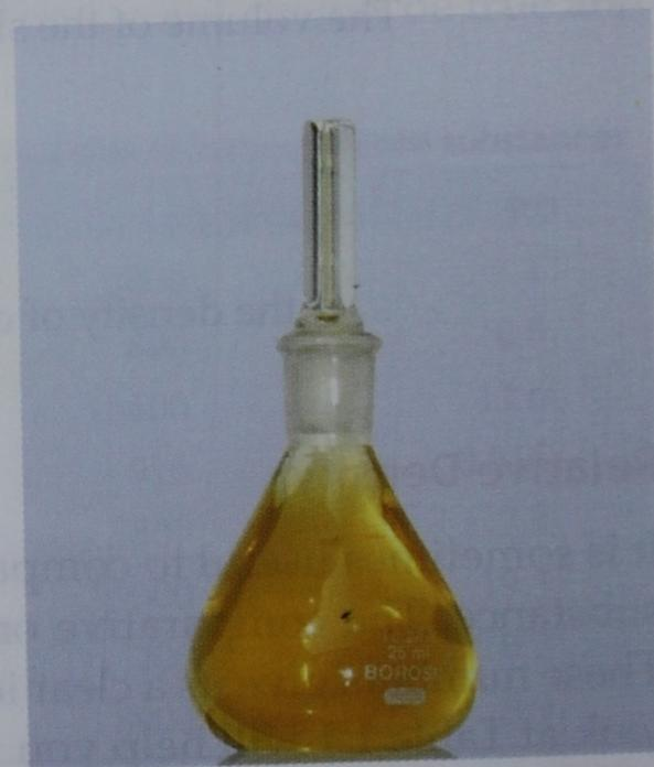
Fig. 1.4 Specific gravity bottle
