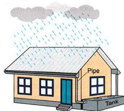
Fig. 5.10 Rooftop rainwater harvesting
