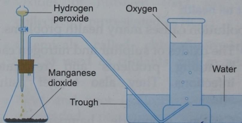
Fig. 4.1 The preparation of oxygen
