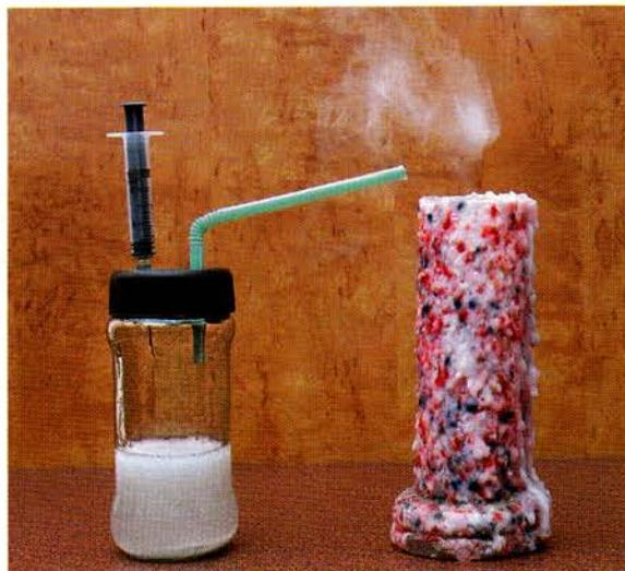
To make a fire extinguisher, you would need a jar with a plastic cap (about the size of a 50-g coffee jar), a 2-mL disposable syringe, a drinking straw that bends at the neck, baking soda and hydrochloric acid used for cleaning bathrooms.
