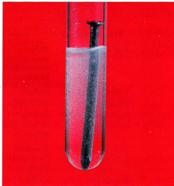
Fig. 3.4 Iron reacts with dilute sulphuric acid to form hydrogen gas and a green solution of iron(II) sulphate.
