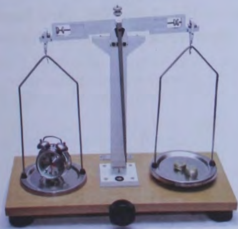
Fig. 1.14 A physical balance
