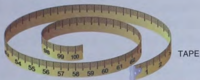
Fig. 1.4 Big lengths are measured with the help of a measuring tape
