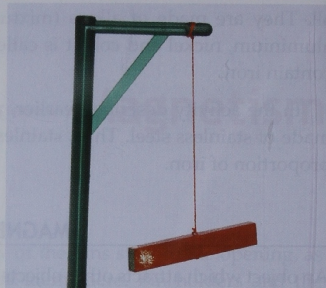
Fig. 6.4 A magnet which can rotate freely comes to rest along the north–south direction.
