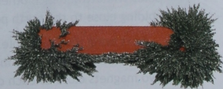
Fig. 6.3 Iron filings are attracted mostly by the two ends of a bar magnet.
