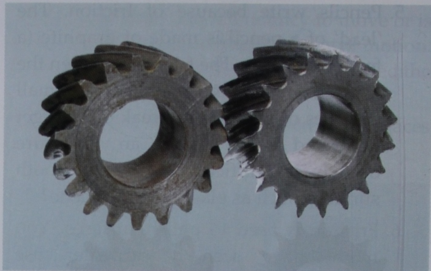
Fig. 3.10 The teeth of the gear on the right have worn out (become thinner) due to friction.
