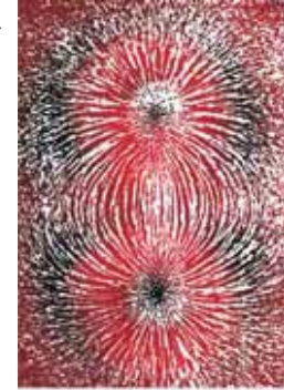
Figure 5.2 Systematic Arrangement of Iron Filings Representing Magnetic Field Lines of a Bar Magnet
