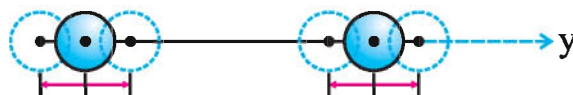
The vibration of the atoms of diatomic molecule about their mean position along the line ( y ) joining them
