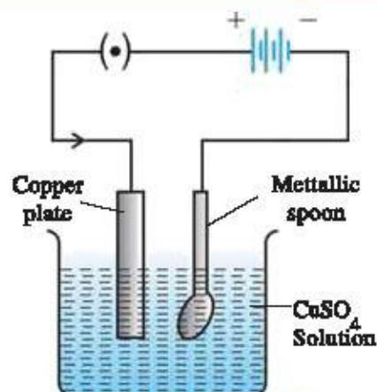
Fig. 4.16 Electroplating
