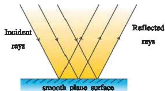
Fig. 2.2 Regular reflection of light
