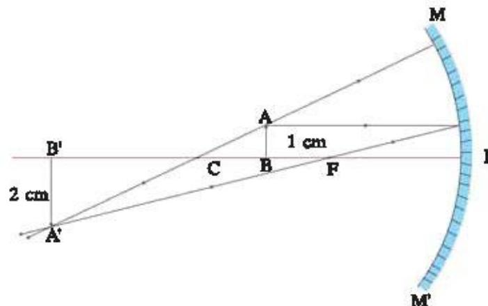
Fig. 2.10.1 (Ray diagram) Image formation by concave mirror
