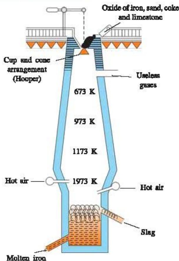
Fig. 8.6 Blast furnace
