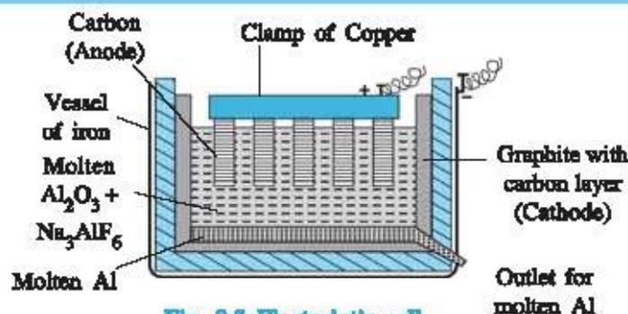
Fig. 8.5 Electrolytic cell
