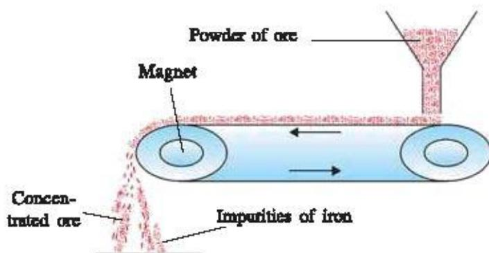
Fig. 8.2 Magnetic separation
