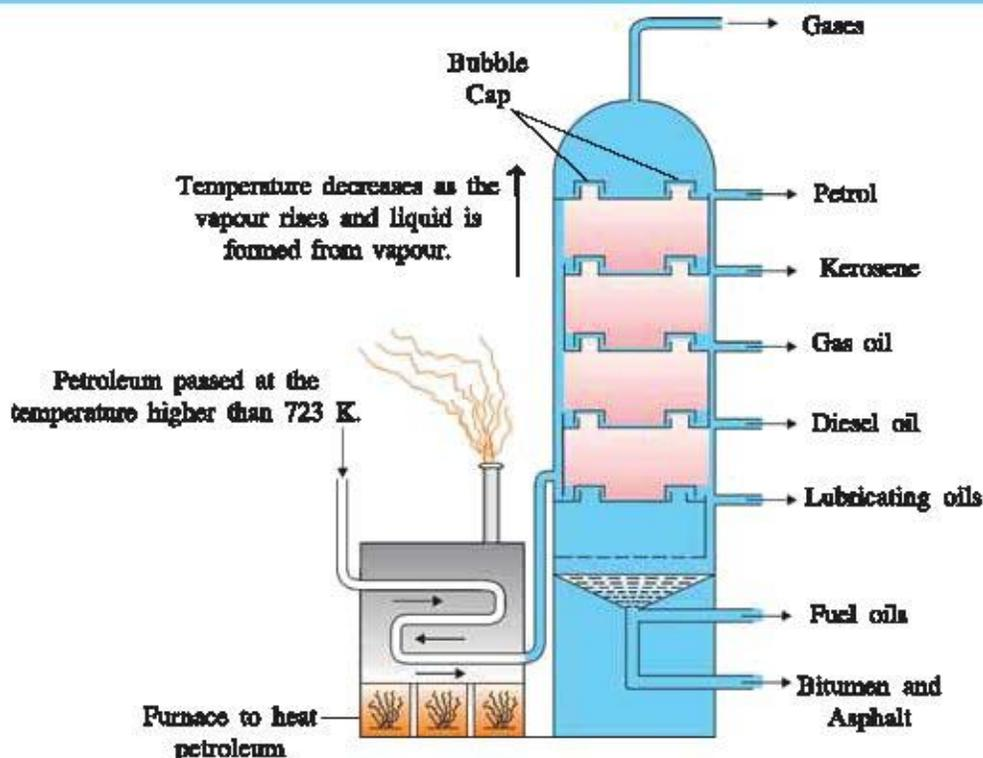
Fig. 10.2 Distillation Tower
