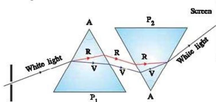
Fig. 3.2 Recombination of spectrum of white light
