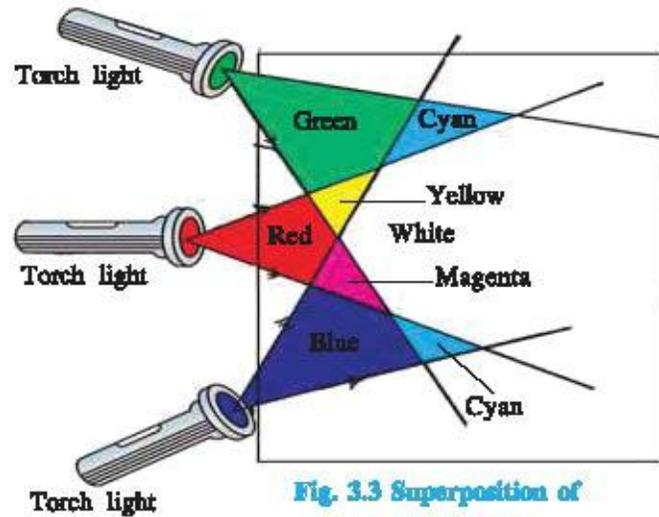
Fig. 3.3 Superposition of primary colours
