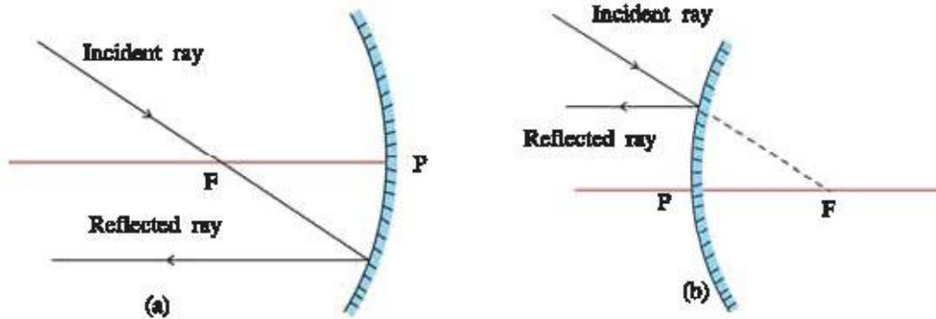
**Fig. 2.8 (a) Ray passing through principal focus of concave mirror
