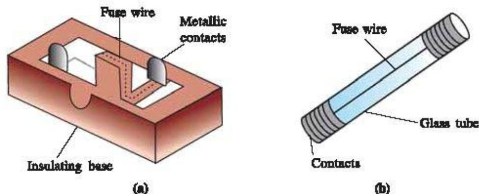
Fig. 5.17 Fuse construction
