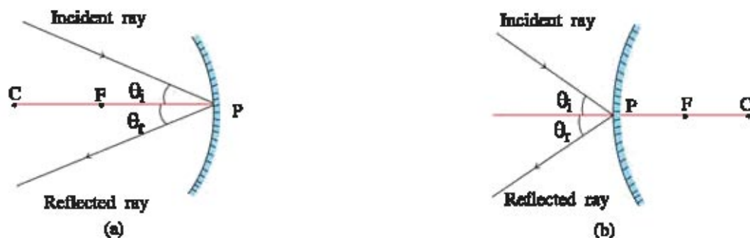
Fig. 2.10 a ray incident obliquely to principal axis towards pole of a mirror
