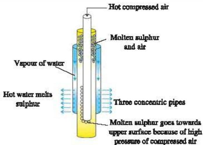
Fig. 9.2 Frasch method for production of sulphur
