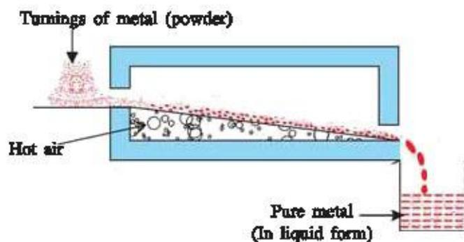
Fig. 8.4 Refining of metal by liquefaction method
