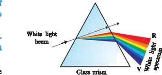
Fig. 3.1 Dispersion of white light by the glass prism.
