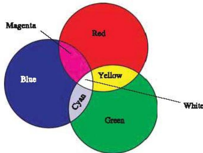
Fig. 3.4 Mixing of primary colours of light
