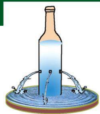
Fig. 3.7 Liquid exerts equal pressure on the walls at equal depths.
