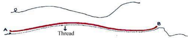
Figure 6.7 Measuring the length of an arc
