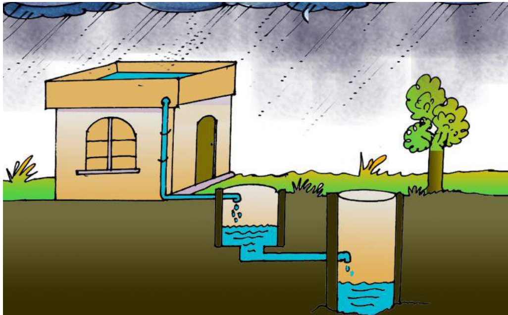
Fig 2.3 Rooftop rain water harvesting
