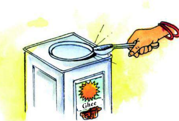
Fig. 11.7 Spoon in the form of a lever
