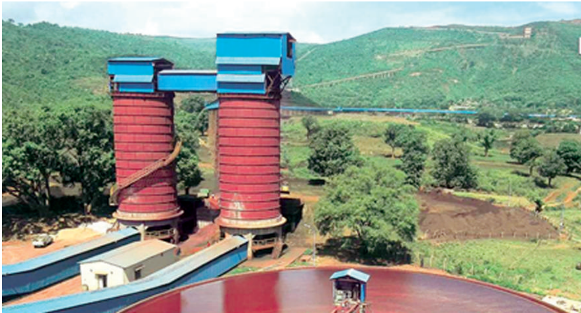
Figure 4.6 : Part of Dantebada-Visakhapatnam Slurry Line - Here the iron ore solution is made
