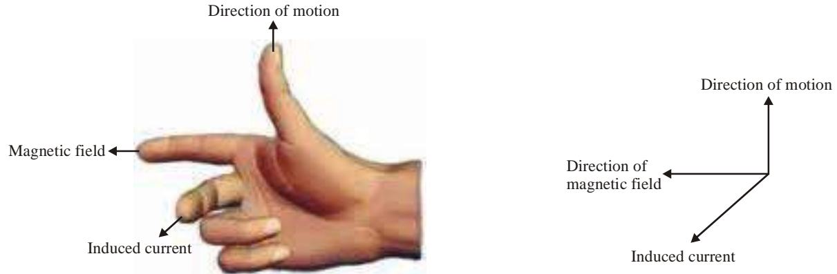
Figure-15: Fleming's right hand rule
