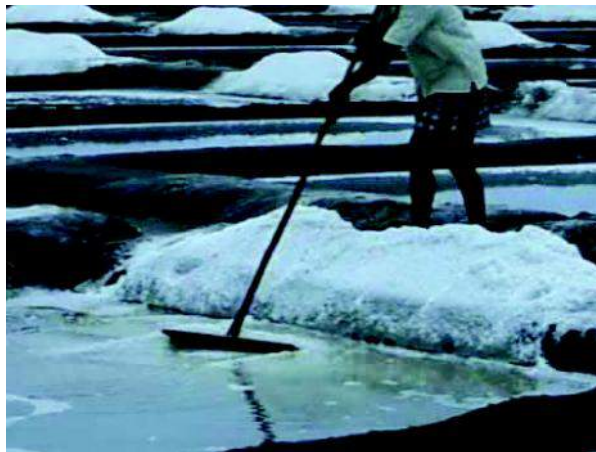
Figure-1: Production of salt from sea water
