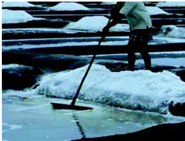
Figure-1: Production of salt from sea water
