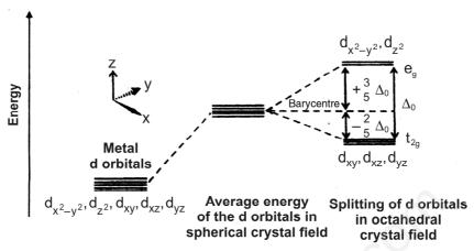
d orbitals splitting in an octahedral crystal-field
